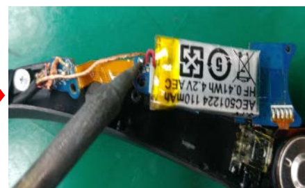
Remove battery wire.
