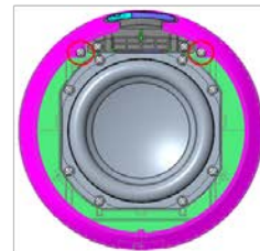
4) Disassemble of the Jersey Assy (2 screw)
