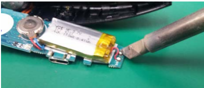
Remove battery wire.
