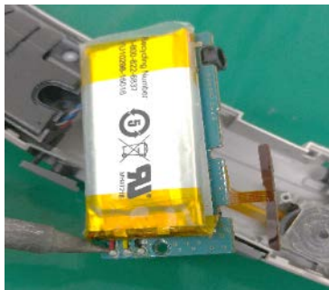
Remove battery wire.
