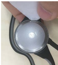
Using a tool, detach Upper case.
