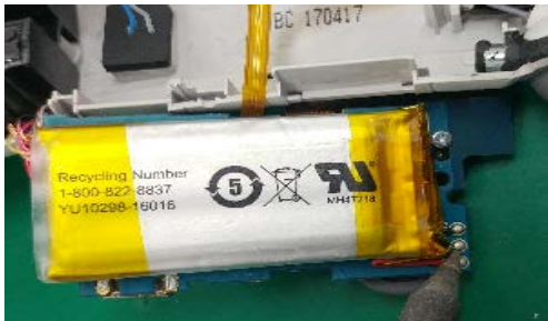
Remove battery wire.
