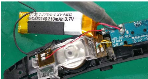
Remove battery wire.
