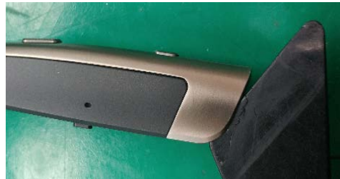
Insert the tool to the edge, and then disassemble from right to left .
