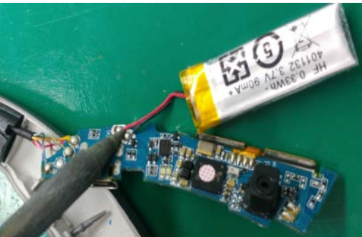
Remove battery wire.
