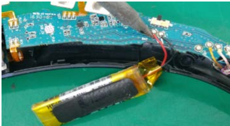
Remove battery wire.
