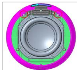
3) Disassemble of the Jersey Assy (2 screw)
