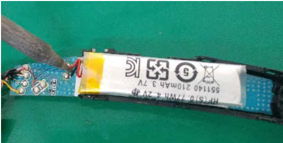
Remove battery wire.
