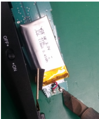
Remove battery wire.
