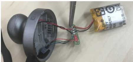
Remove battery wire.
