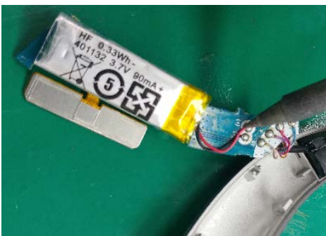
Remove battery wire.
