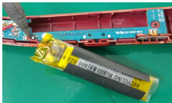
Remove battery wire.
