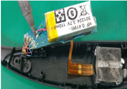
Remove battery wire.
